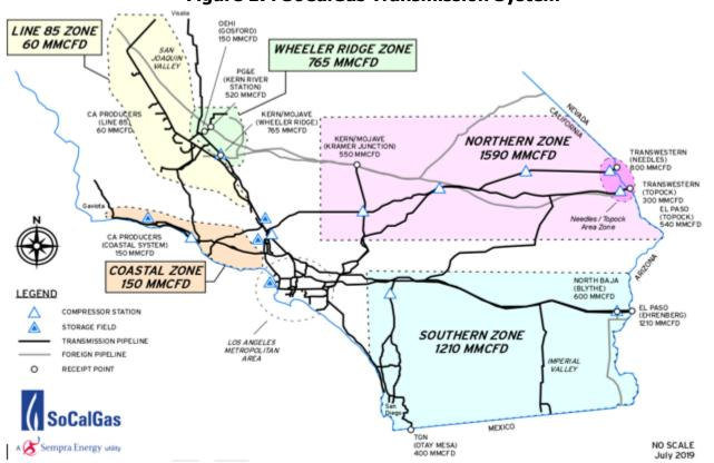
Figure 17: SoCalGas Transmission System
