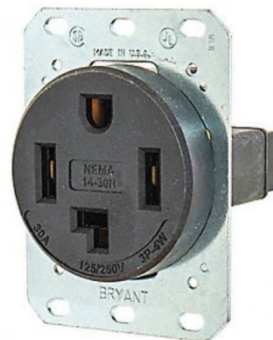
NEMA 14-30 is a four-wire 240v, 30Amp receptacle
