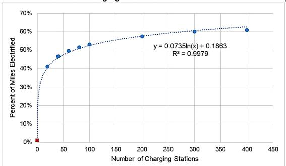
Figure 14: Effect of Slow Charging EVSE on Electrification of Taxi Miles in Beijing
