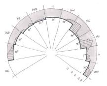
(b) Within each compass sector, the highest altitude angle is selected and used for that entire sector. This datum is shown for a single point of reference on the array.
