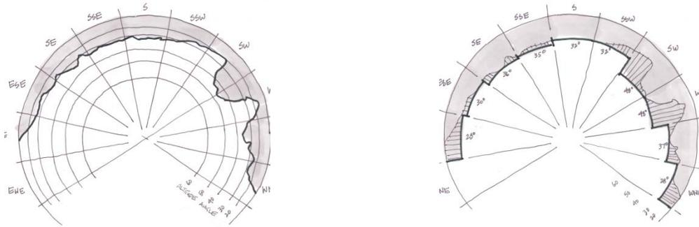
(a) This diagram shows the 22.5° compass sectors used by the PV Calculator and the altitude angles determined by a solar assessment tool for a single point of reference on the array.
