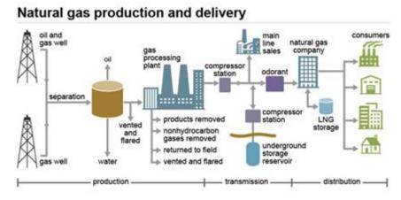
Figure 22: Typical Natural Gas System
