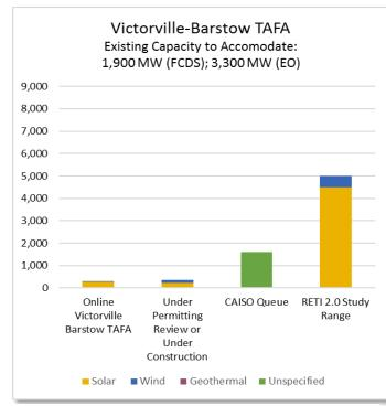
Figure A-10: Victorville-Barstow TAFA Existing and Proposed Renewable Energy and Available Transmission Capacity
