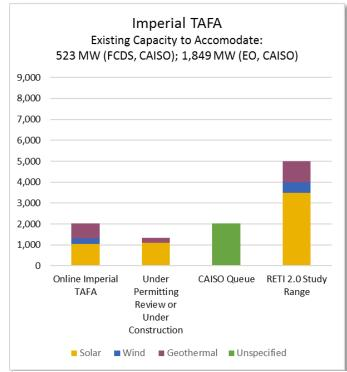
Figure A-6: Imperial Valley TAFA Existing and Proposed Renewable Energy and Available Transmission Capacity
