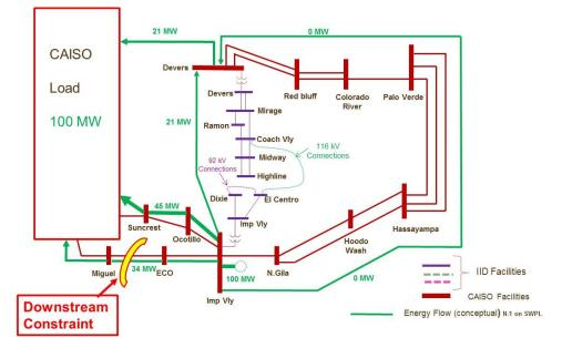
Figure 3-8: Impact of 100 MW Generator Interconnected at Imperial Valley Substation on Downstream Constraint
