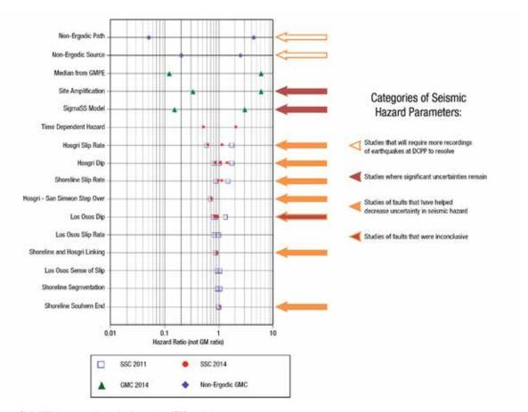
Figure 54: Seismic Hazard Categories at Diablo Canyon
