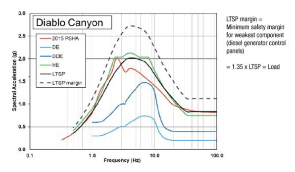
2015 PSHA = PG&E March 2015; DE = Design Earthquake; DDE = Double DE; HE = Hosgri Evaluation; LTSP = 1988 Long Term Seismic Program
