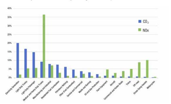
Figure 75: Percentage Contribution of NO<sub>x</sub> and CO<sub>2</sub> Emissions by Different Sources
