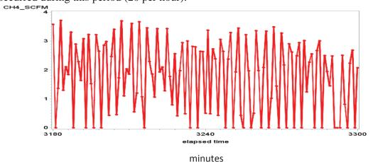
**Figure S1-6.** Methane venting through temporary stack in a water flowback tank for Gulf Coast Completion 1. Six hours of data are shown; 24 discharge events occurred during this period (4 per hour).
