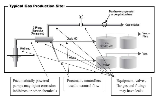
The equipment present on individual well sites can be highly variable. Sites could contain one or multiple wells. Some sites isolate wells from separators and their controllers and in these cases, a site may have no wells. At sites with multiple wells, the wells might each have their own separator and tank system, or separator and tank systems servicing multiple wells might be in place. Additional equipment such as dehydrators and compressors were present on
