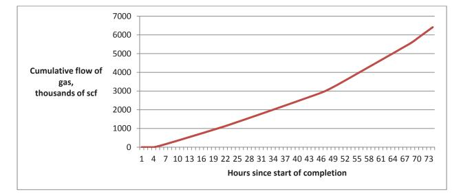
Figure S1-4. Flow of gas from well completion separators to a flare (Gulf Coast Completion 1)
