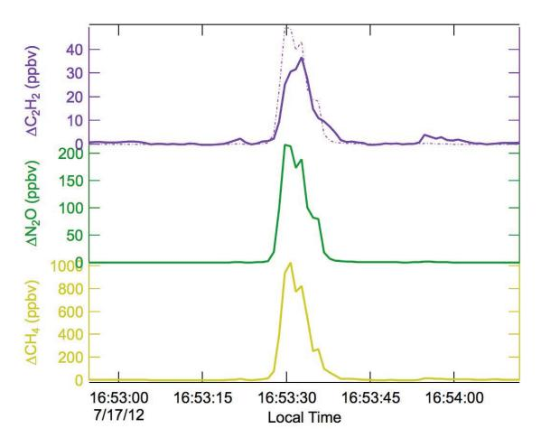
**Figure S4-2.** Acetylene,  $N_2O$  and methane concentration profiles (background corrected) along the path traversed by the measurement van (horizontal axis is local measurement time). Also shown is a hypothetical distribution of acetylene (dashed blue line) that would be anticipated, if the releases were co-located.
