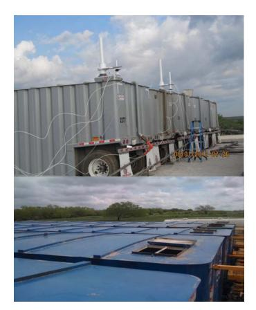
**Figure S1-3.** Oil and water flowback tanks. Upper and middle: Hatches in the tanks allowed gases to vent to the atmosphere; temporary stacks were installed on the hatches to measure gas flow. Samples for gas composition analyses were drawn from the stack, through tubing, to a remote sampling port.
