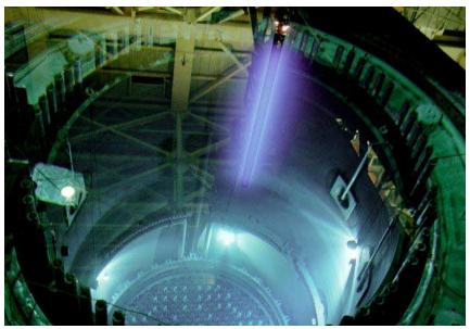
A nuclear fuel assembly being removed from the reactor at the Columbia Generating Station in Richland, WA during a refueling outage. The blue glow results from Cherenkov radiation, emitted as subatomic particles from the fuel move through the water faster than the phase velocity of light. Source: Energy Northwest
