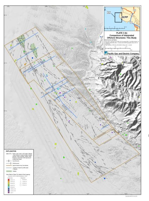
Connection between Shoreline and Hosgri faults demonstrated by Point Buchon 3-D seismic survey.
