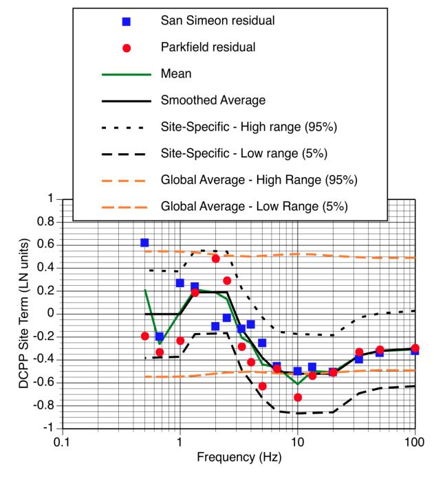
An empirical site amplification factor has been developed by PG&E to explain relatively low ground motions from the San Simeon 2003 and Parkfield 2004 earthquakes. If this factor is due to some intrinsic properties of the site, then it would apply to any earthquake.
