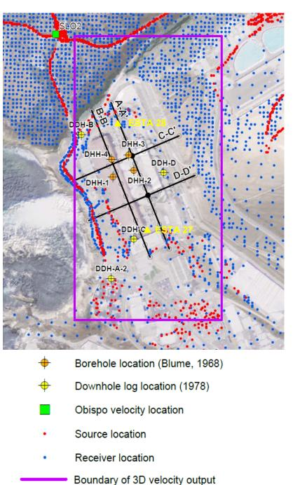
Seismic survey used to develop 3-D velocity model of foundation area and standard "site conditions" where previous earthquakes were recorded.
