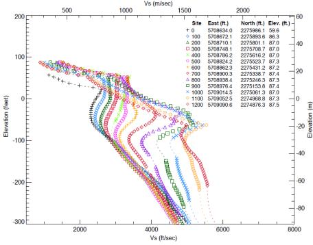
GeoTomo Vs Profile B-B' sites using Vp/Vs depth relation
