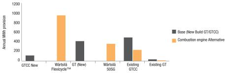
Figure 3. Provision of Regulation Up (RegUp) ancillary service for the two scenarios. Combustion engines provide more than double the amount of RegUp compared to the gas turbine/Base buildout and reduce provision of this A/S by the existing GTs and GTCCs.
