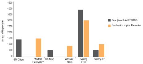
Figure 4. Provision of Spinning Reserve (Spin) ancillary service for the two scenarios. Simple cycle combustion engines provide double the amount Spin compared to the GTs in the Base scenario.
