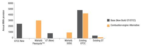
Figure 2. Provision of Load Following Up (LFUP) ancillary service for the two scenarios. Combustion engines provide 30% more LFUP than the gas turbine/Base buildout, and reduce provision of LFUP by the existing GTs and GTCCs.
