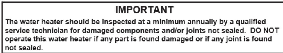
Figure 8: Storage Water Heater Maintenance Recommendation
