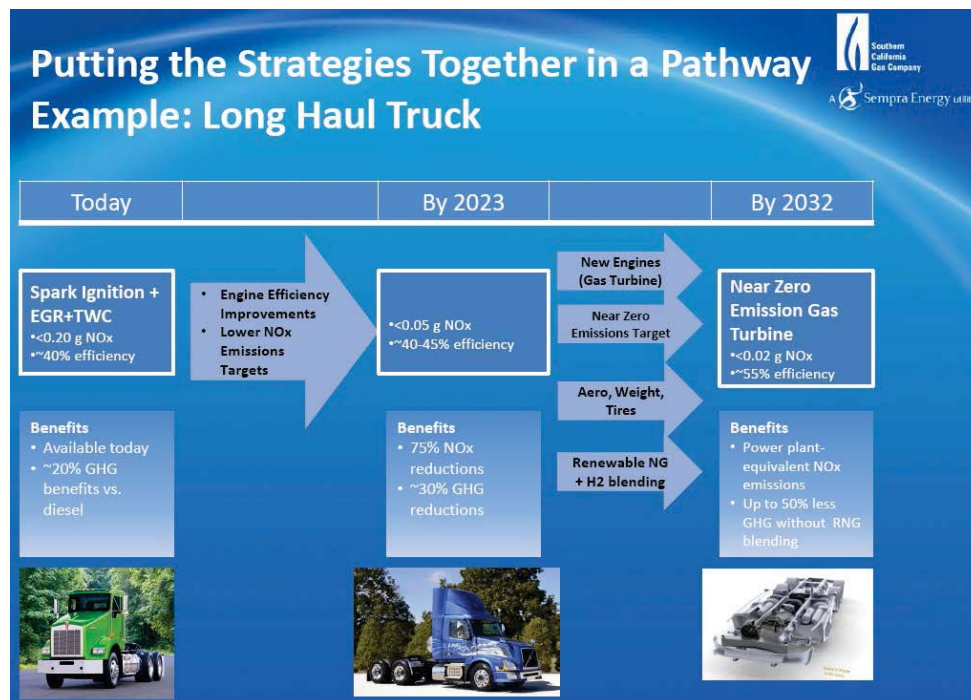
Figure 27: NO x and Carbon Emission Reduction Strategies for a Long-Haul Truck
