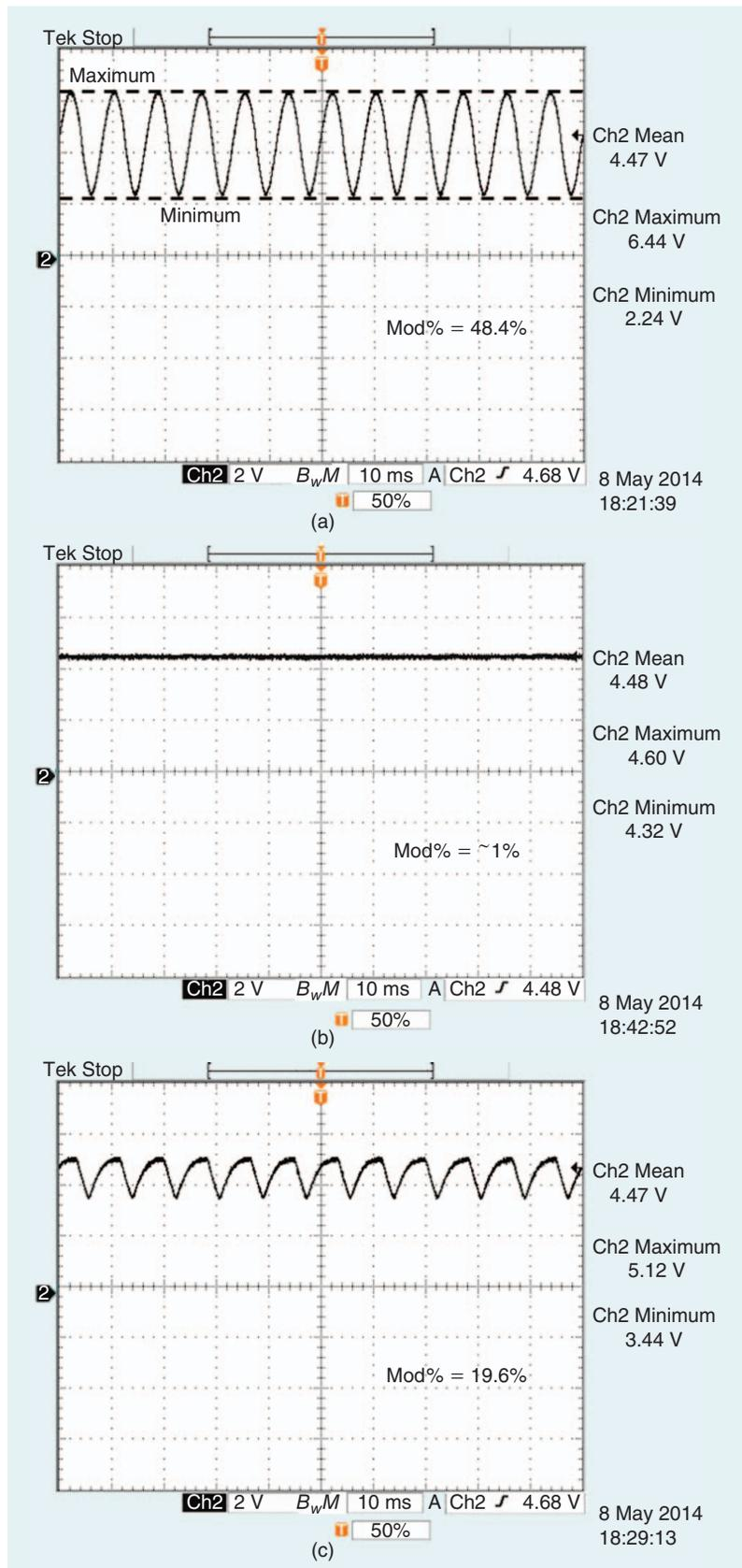
**FIG 2** The typical plots of luminance light flicker in commercial LED A19 bulbs (60-W incandescent replacement bulbs).  $\text{Mod}\% = (\text{Max luminance} - \text{Min luminance}) / (\text{Max luminance} + \text{Min luminance})$ .  $\text{Mod}\%$  for the three bulbs are (a) Utilitech, 48.4%; (b) Philips, <1%; and (c) GE, 19.6%.
