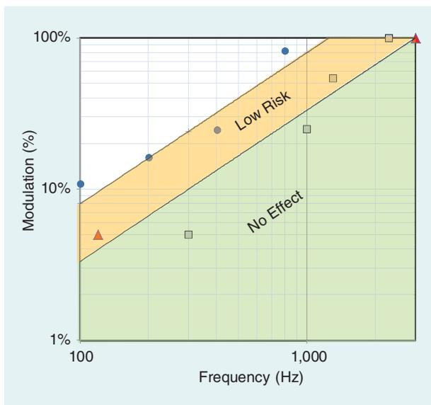
**FIG 6** The low-risk (orange) and no-observable-effect (green) regions for flicker as a function of the frequency and modulation percentage. The line  $\text{Mod}\% = 0.0333 \cdot f_{\text{Flicker}}$  separates the no-observable-effect and low-risk regions, and the upper margin of the low-risk region is given by the line  $\text{Mod}\% = 0.08 \cdot f_{\text{Flicker}}$ . (Data taken from Figure 3 of [14] and [15].)
