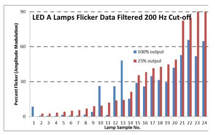
Figure 4: Filtered Flicker Test Data for 25 LED A-lamps (filtered flicker proposed for CA standards)
