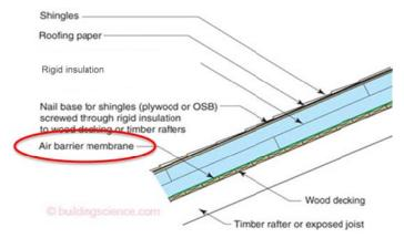
Figure 10: Moisture Management in Above Roof Deck Insulation (BSC)
