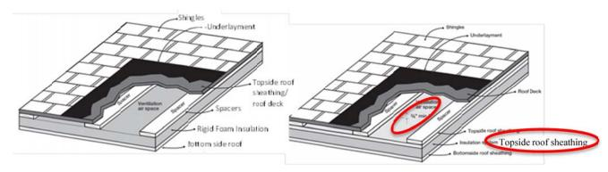
Figure 8: Ventilation for Asphalt Shingles (ARMA Form No. 211-RR-94 2008)
