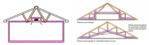
Figure 3: Options for Conditioned Plenum Space (adopted from Ductsinside.org and **CEC 2003c)**
