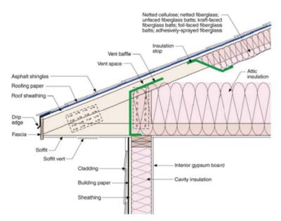
Figure 15: Venting Details for Modified Conventional Vented Attic
