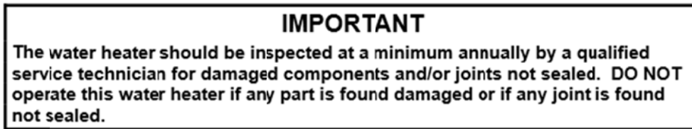
Figure 5: Storage Water Heater Maintenance Recommendation
