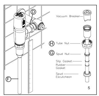
**5.)** Determine the length of vacuum breaker tube **(F)** required to join the flush valve and fixture spud. Cut the vacuum breaker tube, if required, to this length. Assemble the vacuum breaker tube assembly and spud nut assembly to the flush valve and fixture spud.
