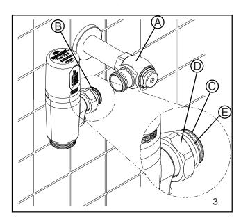
3.) Prior to inserting the flush valve tailpiece (B) into stop valve (A), be certain that the O-ring seal (C) is located in O-ring seal groove at the end of the tailpiece and that the locking nut (D) and locking snap ring (E) are located as shown. Care should be taken not to damage the O-ring when inserting the tailpiece into the stop valve. If lubrication is needed, wetting the O-ring with water will be sufficient.
