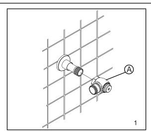
Install stop valve assembly (A) using proper size supply escutcheon and sweat solder adapter kit if applicable.
