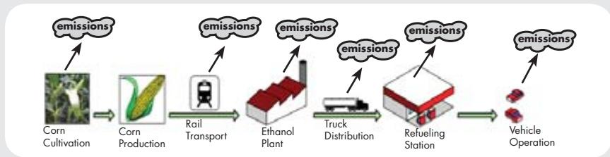
*A fuel life-cycle analysis traces a fuel pathway from well to wheels. The corn ethanol pathway is shown here as an example. Source: M. A. Delucchi, Lifecycle Analyses of Biofuels (Institute of Transportation Studies, University of California, Davis, 2006), UCD-ITS-RR-06-08.*
