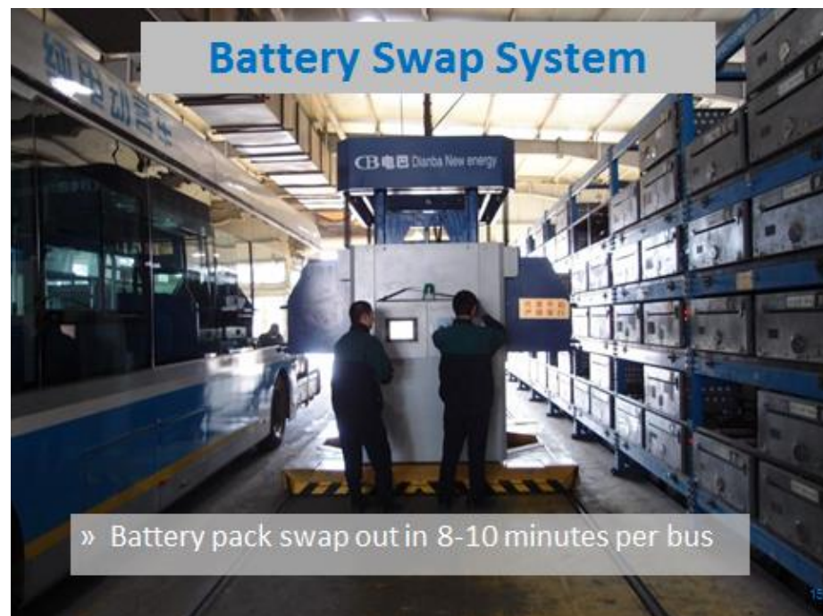
Figure 3.12 Battery Swapping for Transit Buses, China
