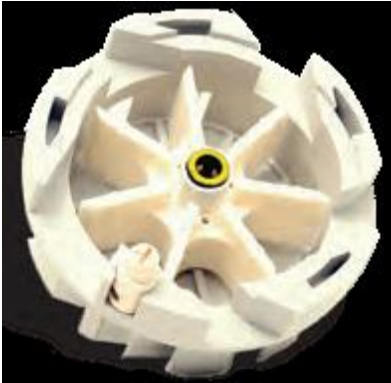
Figure 5: Photograph of multi-jet meter measuring chamber
