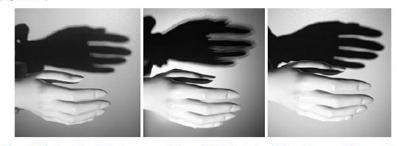
Figure 1-3 Shadows from (left) a large source (Halogen MR16), (center) multiple point sources (first generation LED MR 16 with 4 LEDs) and (right) single point source (GaN on GaN LED MR16) source
