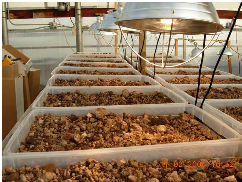
Figure 2-9. Treated Arizona Soil Trays Under the Heat Lamps
