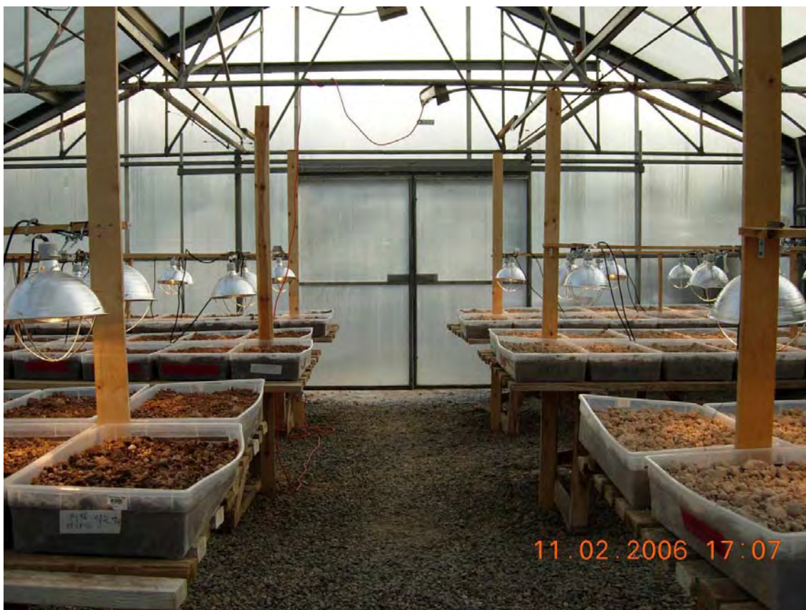
Figure 2-8. Greenhouse (AZ soils on the left, NV soils on the right) under heat lamps
