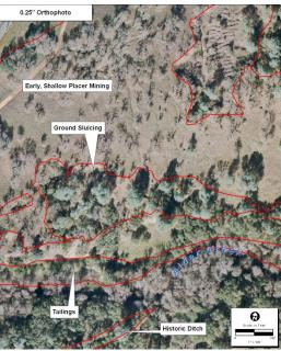
EXHIBIT 624. LIDAR imagery (left) compared to aerial imagery. Notice the clearly visible areas of ground sluicing and early shallow, placer mining, as well as the ditches.
