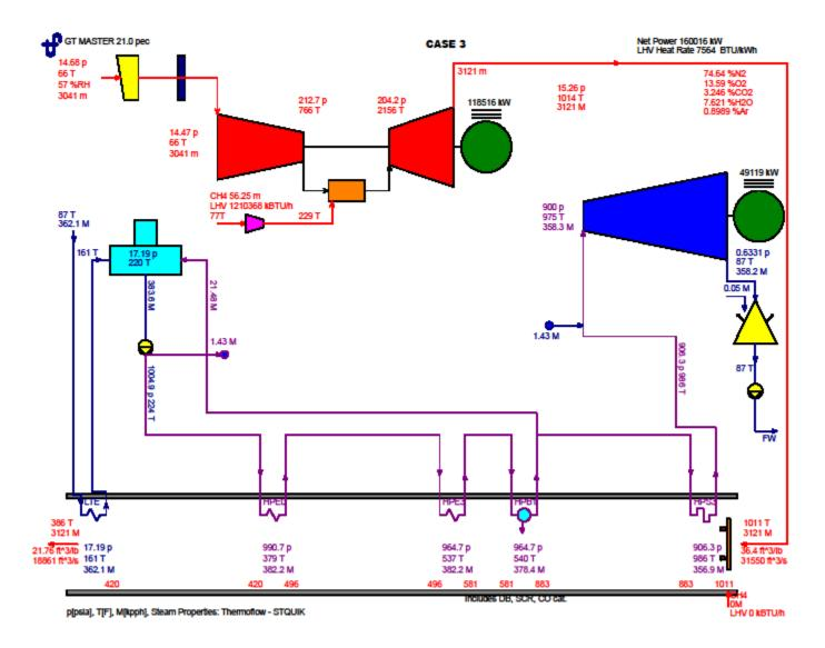
Case 3 Heat Balance Number 1c One Combustion Turbine Operating at Maximum Heat Input without Evaporative Cooling Site Average Annual Temperature (SAAT), Dry Bulb 65.8 F, Wet Bulb 56.8 F, Relative Humidity 57%
