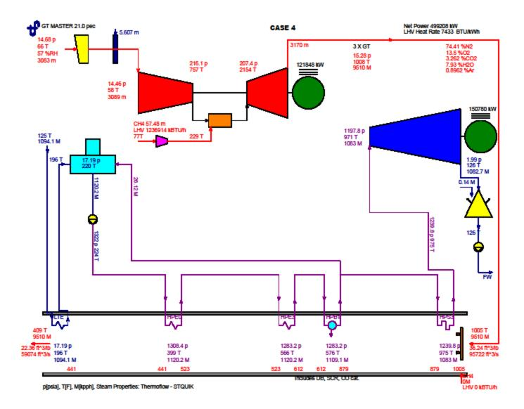
Case 4 Heat Balance Number 2a Three Combustion Turbines Operating at Maximum Heat Input with Evaporative Cooling Site Average Annual Temperature (SAAT), Dry Bulb 65.8 F, Wet Bulb 56.8 F, Relative Humidity 57%
