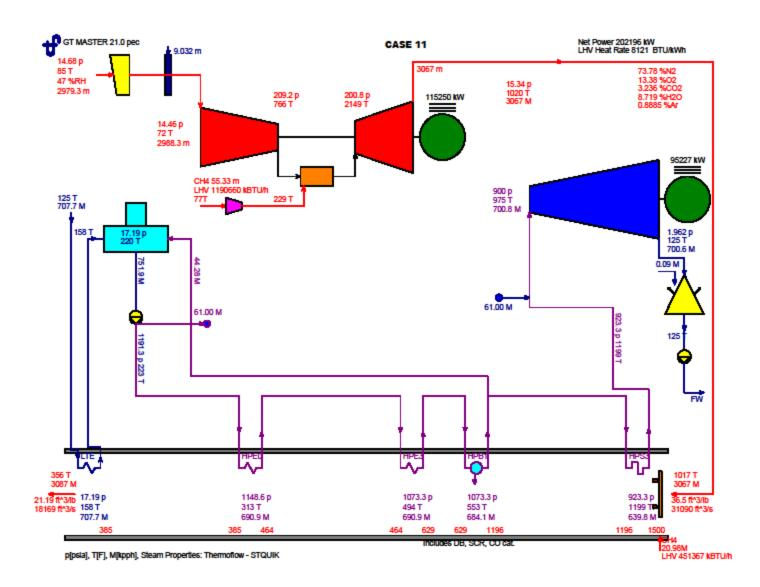
Case 11 Heat Balance Number 3c(1) One Combustion Turbine Operating at Maximum Heat Input with Evaporative Cooling and Duct Burning Site Monthly Maximum Average Ambient Temperature (SMMAAT) is 85 °F (Dry Bulb) and 69.7 °F (Wet Bulb) and relative humidity (RH) of 45.75%) Case 11 Heat Balance Number 3c(1)
