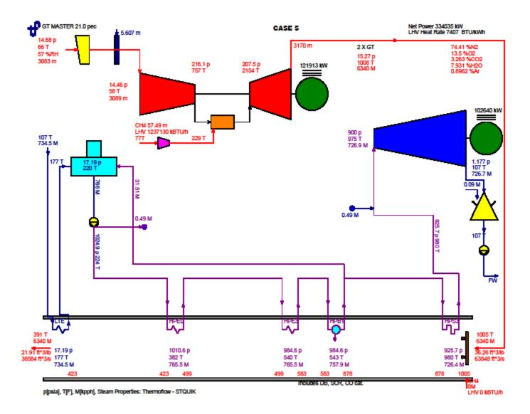
Case 5 Heat Balance Number 2b Two Combustion Turbines Operating at Maximum Heat Input with Evaporative Cooling Site Average Annual Temperature (SAAT), Dry Bulb 65.8 F, Wet Bulb 56.8 F, Relative Humidity 57%
