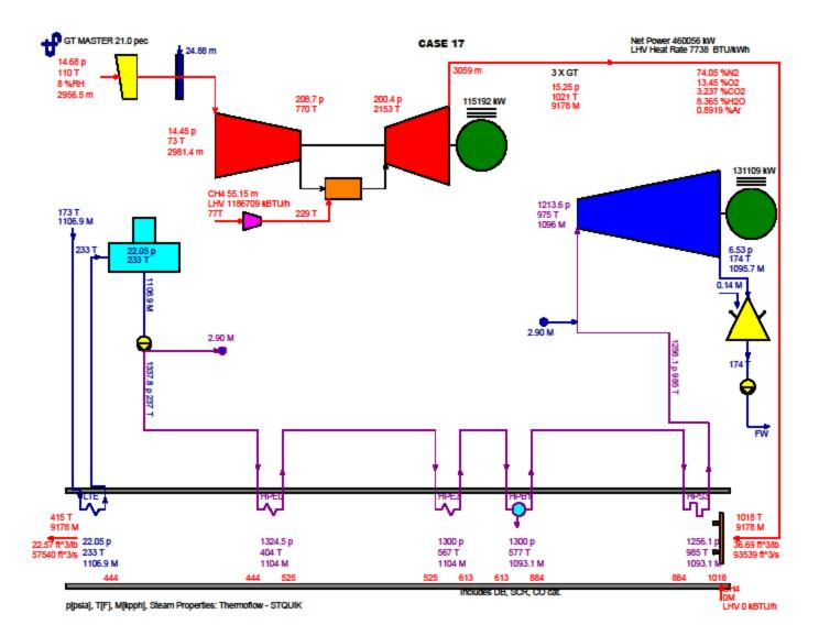
Case 17 Heat Balance Number 6 Three Combustion Turbines Operating at Maximum Heat Input with Evaporative Cooling Site Peak Summer Ambient Temperature (SPSAT) is 110 °F (Dry Bulb) and 67 °F (Wet Bulb) and relative humidity (RH) of 7.31%)
