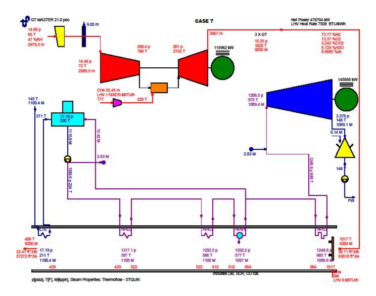
Case 7 Heat Balance Number 3a Three Combustion Turbines Operating at Maximum Heat Input with Evaporative Cooling Site Monthly Maximum Average Ambient Temperature (SMMAAT) is 85 °F (Dry Bulb) and 69.7 °F (Wet Bulb) and relative humidity (RH) of 45.75%)
