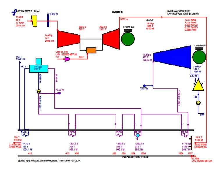
Case 9 Heat Balance Number 3b(1) Two Combustion Turbines Operating at Maximum Heat Input with Evaporative Cooling and Duct Burner Site Monthly Maximum Average Ambient Temperature (SMMAAT) is 85 °F (Dry Bulb) and 69.7 °F (Wet Bulb) and relative humidity (RH) of 45.75%)
