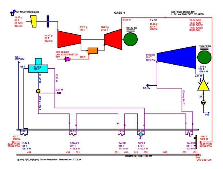
Case 1 Heat Balance Number 1a Three Combustion Turbines Operating at Maximum Heat Input without Evaporative Cooling Site Average Annual Temperature (SAAT), Dry Bulb 65.8 F, Wet Bulb 56.8 F, Relative Humidity 57%
