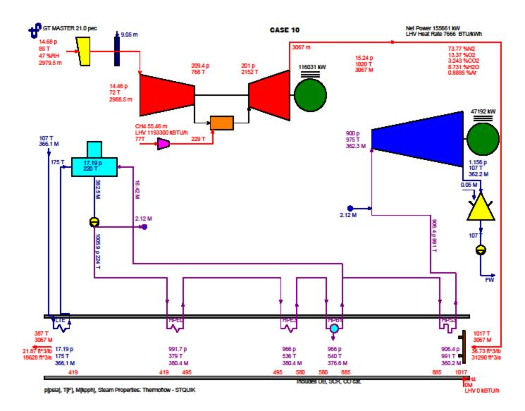
Case 10 Heat Balance Number 3c One Combustion Turbine Operating at Maximum Heat Input with Evaporative Cooling Site Monthly Maximum Average Ambient Temperature (SMMAAT) is 85 °F (Dry Bulb) and 69.7 °F (Wet Bulb) and relative humidity (RH) of 45.75%)
