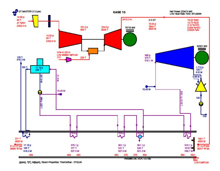
Case 13 Heat Balance Number 4b Two Combustion Turbines Operating at Minimum Heat Input without Evaporative Cooling Site Monthly Maximum Average Ambient Temperature (SMMAAT) is 85 °F (Dry Bulb) and 69.7 °F (Wet Bulb) and relative humidity (RH) of 45.75%)
