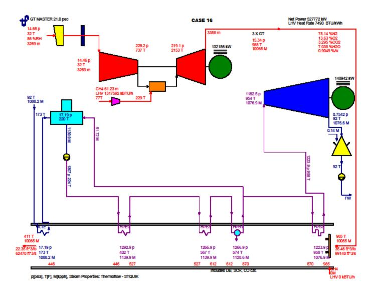
Case 16 Heat Balance Number 5 Three Combustion Turbines Operating at Maximum Heat Input without Evaporative Cooling Site Minimum Winter Ambient Temperature (SMWAT) is 32 °F (Dry Bulb) and 30.75 °F (Wet Bulb) and relative humidity (RH) of 87.6%)
