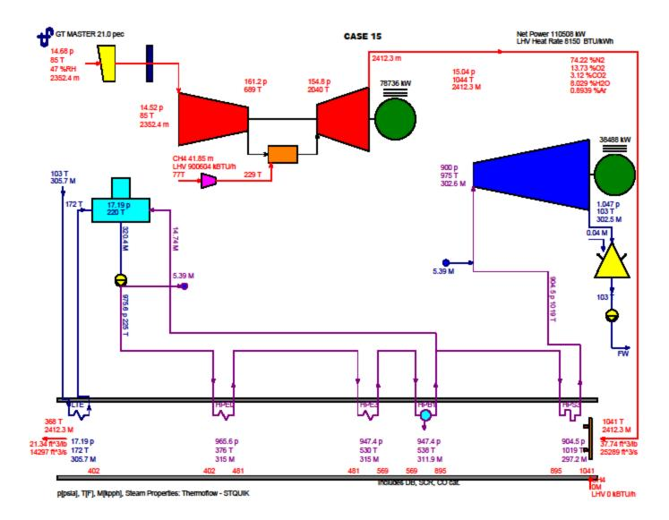
Case 15 Heat Balance Number 4c One Combustion Turbine Operating at Minimum Heat Input without Evaporative Cooling Site Monthly Maximum Average Ambient Temperature (SMMAAT) is 85 °F (Dry Bulb) and 69.7 °F (Wet Bulb) and relative humidity (RH) of 45.75%)
