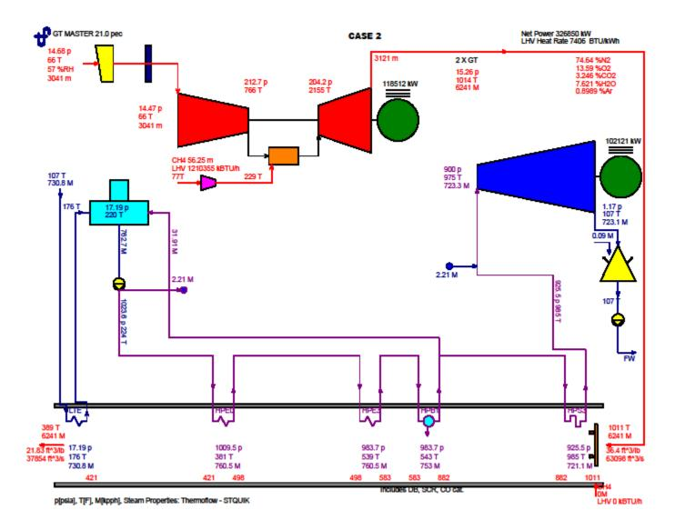
Case 2 Heat Balance Number 1b Two Combustion Turbines Operating at Maximum Heat Input without Evaporative Cooling Site Average Annual Temperature (SAAT), Dry Bulb 65.8 F, Wet Bulb 56.8 F, Relative Humidity 57%
