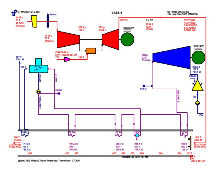
Case 8 Heat Balance Number 3b Two Combustion Turbines Operating at Maximum Heat Input with Evaporative Cooling Site Monthly Maximum Average Ambient Temperature (SMMAAT) is 85 °F (Dry Bulb) and 69.7 °F (Wet Bulb) and relative humidity (RH) of 45.75%)
