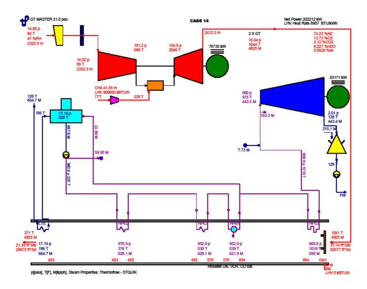
at Balance Number 4b(1) Two Combustion Turbines Operating at Minimum Heat Input without Evaporative Cooling w. portion of HRSG steam sent to ACC Site Monthly Maximum Average Ambient Temperature (SMMAAT) is 85 'F (Dry Bulb) and 69.7 'F (Wet Bulb) and relative humidity (RH) of 45.75%) Case 14 Heat Balance Number 4b(1)
