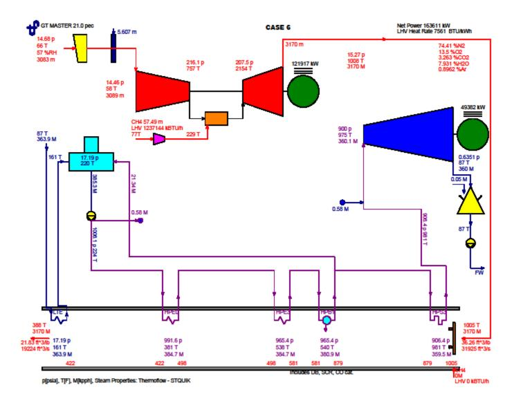
Case 6 Heat Balance Number 2c One Combustion Turbine Operating at Maximum Heat Input with Evaporative Cooling Site Average Annual Temperature (SAAT), Dry Bulb 65.8 F, Wet Bulb 56.8 F, Relative Humidity 57%
