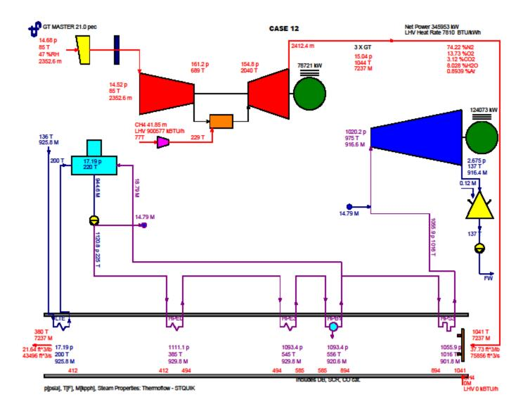
Case 12 Heat Balance Number 4a Three Combustion Turbines Operating at Minimum Heat Input without Evaporative Cooling Site Monthly Maximum Average Ambient Temperature (SMMAAT) is 85 °F (Dry Bulb) and 69.7 °F (Wet Bulb) and relative humidity (RH) of 45.75%)
