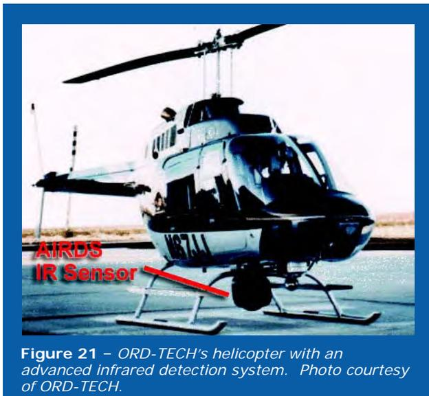
Figure 21 – ORD-TECH's helicopter with an advanced infrared detection system. Photo courtesy of ORD-TECH.
