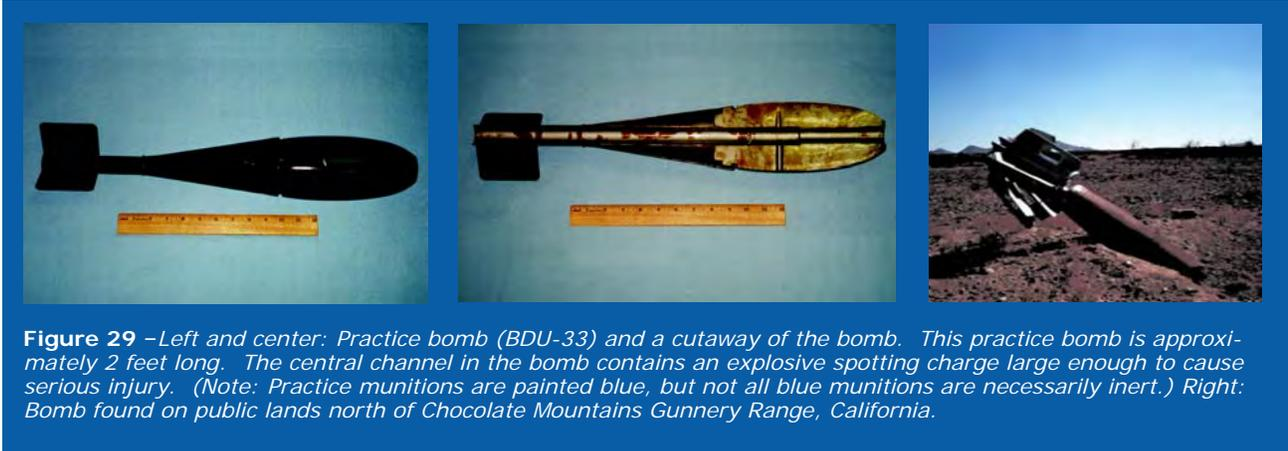
**Figure 29** –Left and center: Practice bomb (BDU-33) and a cutaway of the bomb. This practice bomb is approximately 2 feet long. The central channel in the bomb contains an explosive spotting charge large enough to cause serious injury. (Note: Practice munitions are painted blue, but not all blue munitions are necessarily inert.) Right: Bomb found on public lands north of Chocolate Mountains Gunnery Range, California.
