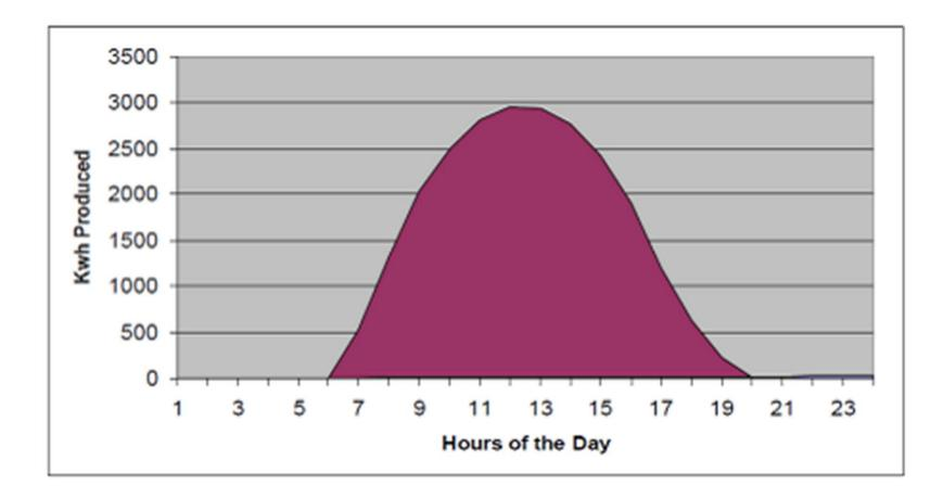
Distributed PV has predictable pattern on partly cloudy days. No fast-response ramping resources necessary. There are 15,000 PV sites in San Diego spread over 100s of square miles (graphic: LBNL)
