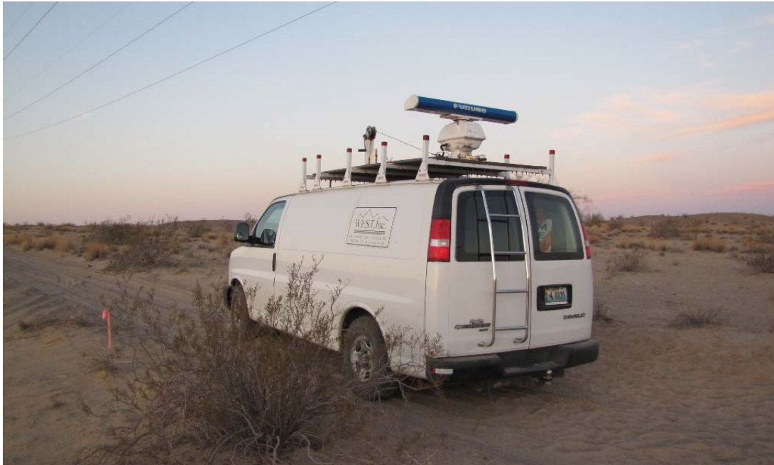
Photo A. Radar van parked at sampling location at the Rio Mesa Solar Electric Generating Facility Radar Study Area. Antenna is in horizontal mode.
