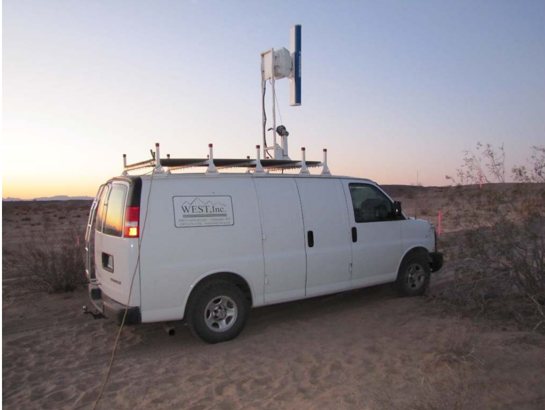
Photo B. Radar van parked at sampling location at the Rio Mesa Solar Electric Generating Facility Radar Study Area. Antenna is in vertical mode.
