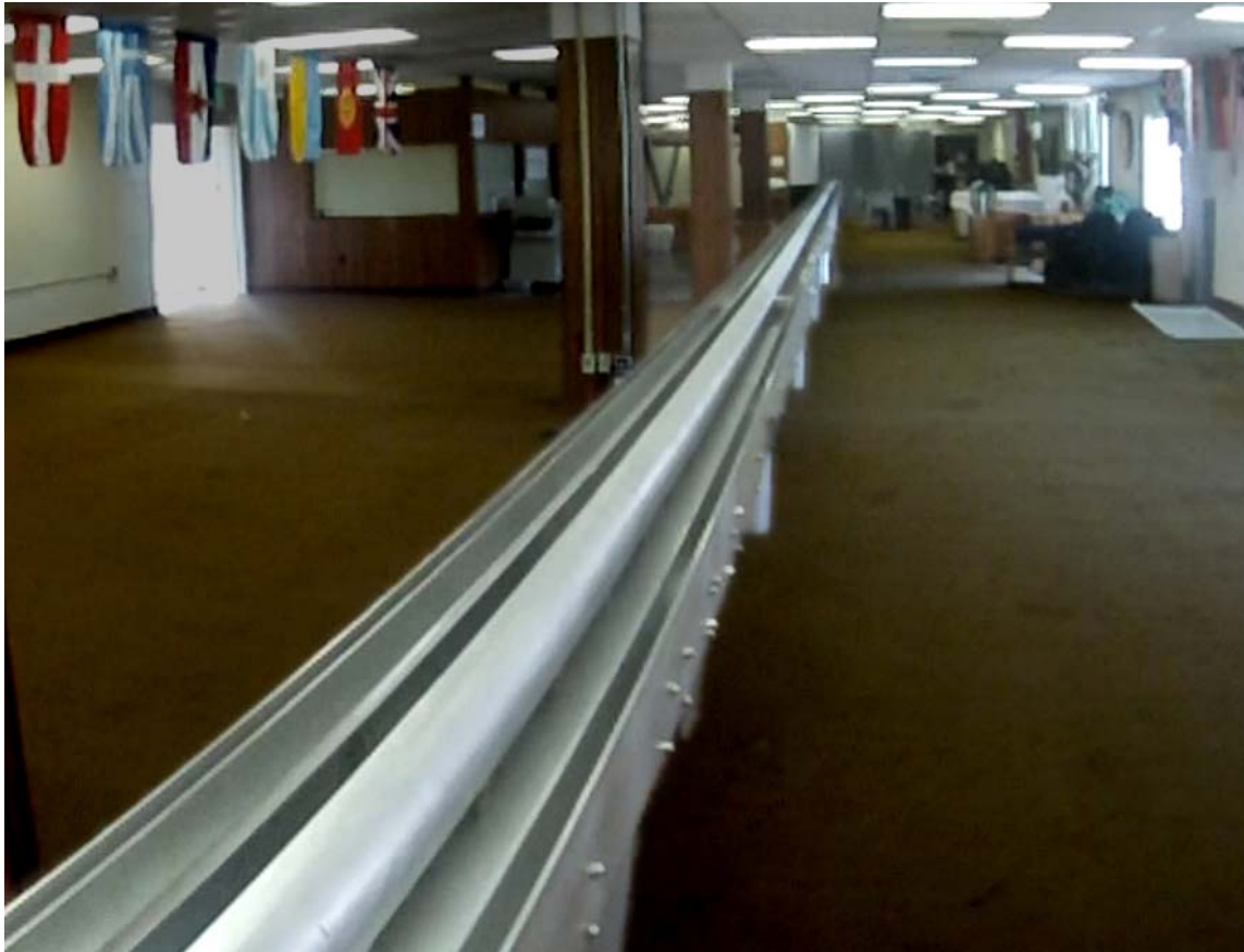
Figure 3a - Magnetic wing sub-scale prototype of guideway NASA Ames Research Center. Guideway has been inverted for testing. The center tube is the reaction tube for the propulsion system. The two outer rails provide a reaction surface for the levitation wings. In full-scale operations, bogie and vehicle hang from guideway.
