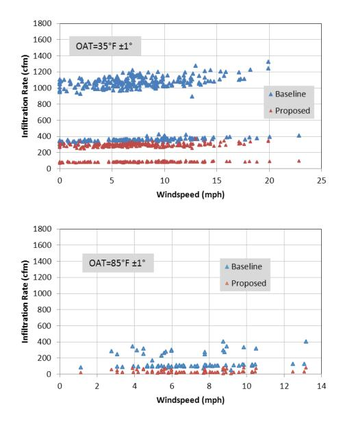
Figure 6 – Infiltration as a Function of Windspeed, Large Office, Bottom Zone 1, Climate Zone 16
