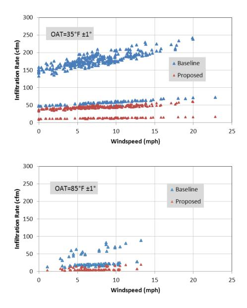
Figure 3 – Infiltration as a Function of Windspeed for the Small Office, Zone 3, Climate Zone 16
