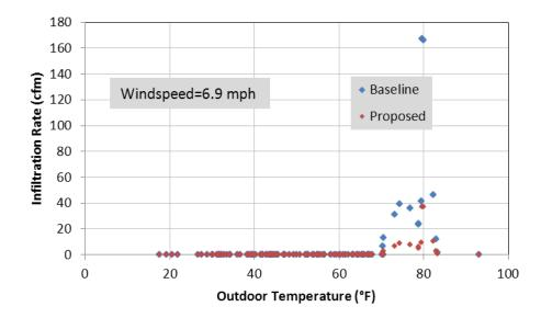
Figure 5 – Infiltration as a Function of Outdoor Temperature for the Large Office, Top Zone 1, CZ 16
