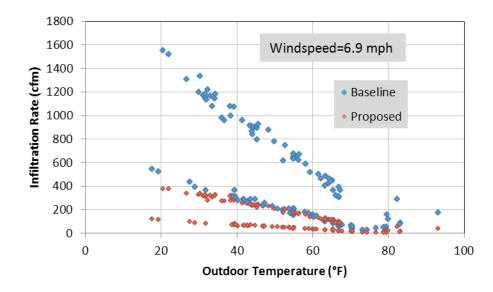
Figure 4 – Infiltration as a Function of Outdoor Temperature for the Large Office, Bottom Zone 1, CZ 16
