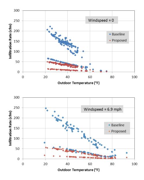
Figure 2 – Infiltration as a Function of Outdoor Temperature for the Small Office, Zone 3, Climate Zone 16
