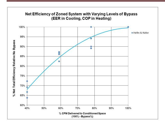
Figure 2. Net Zoned System Efficiency with Bypass (Carrier Lab Data)
