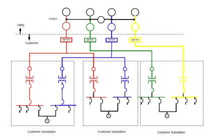
In the diagram above, there is no single site-boundary meter. Instead, the four lines serving the facility, which may have net load or generation, are separately metered by the utility using four separate meters in the same location. The meters are within a few feet, as depicted below.
