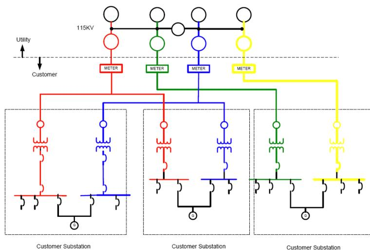
In the diagram above, there is no single site-boundary meter. Instead, the four lines serving the facility, which may have net load or generation, are separately metered by the utility using four separate meters in the same location. The meters are within a few feet, as depicted below.
