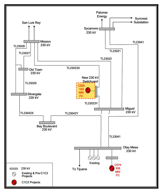
Figure 2.2: Proposed Single Line Diagram
