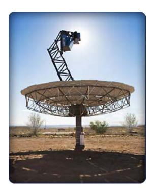
Figure 3.4. Photo of typical SunCatchers<sup>™</sup>.
