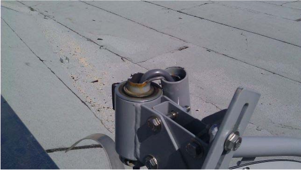
Photo 2 DyoCore Yaw snapped off above the yaw bearing
