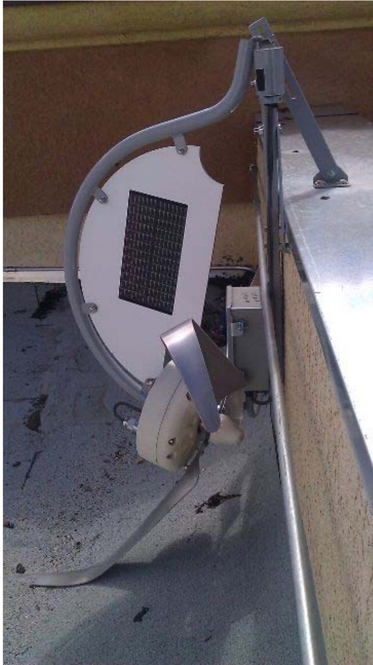
Photo3 Clear view of what is left of the DyoCore turbine
