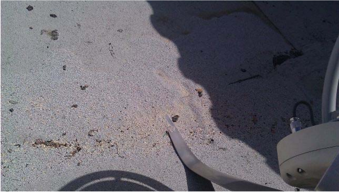
Photo 4 Tip of the blade cuts into roof after yaw assembly broke
