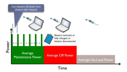
As highlighted, the *Maintenance Power* and the *Off Power* (i.e. *No-Battery Power*) are different. The intent of the *No-Battery* test is to capture a meaningful representation of the power for system functions. For Category 3 devices, the testing procedure does not capture this, and would estimate a much lower power value using *Average No-Load Power*.
