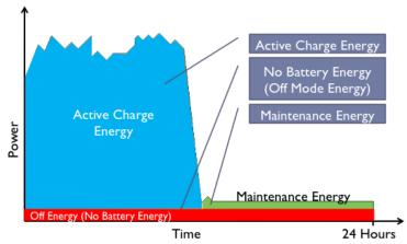
In the current measurement methodology the *Off* energy is captured as part of the Maintenance energy and active charge energy. As the primary function of the device is not battery charging (it's supporting the computer or some other main function) this energy ends up causing the charge efficiency calculations appear low. For a representative value for charging efficiency, *Off* energy should really be subtracted out or accounted for in the limit.
