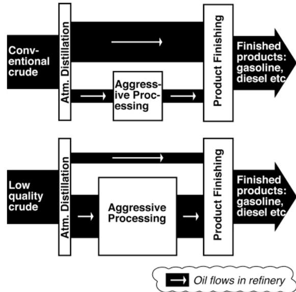
Aggressive processing (vacuum distillation, cracking, and aggressive hydroprocessing) acts on a larger portion of the total crude refined to make motor fuels from lower quality crude, requiring more fuel to be burned for energy and increasing refinery emissions.
