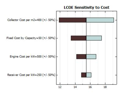
Sensitivity analysis: LCOE is most sensitive to collector cost
