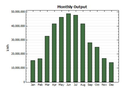
Example: 100 MW Parabolic trough system with 6 hours of storage
