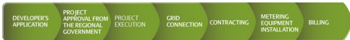
Figure 20: DG Connection Process
