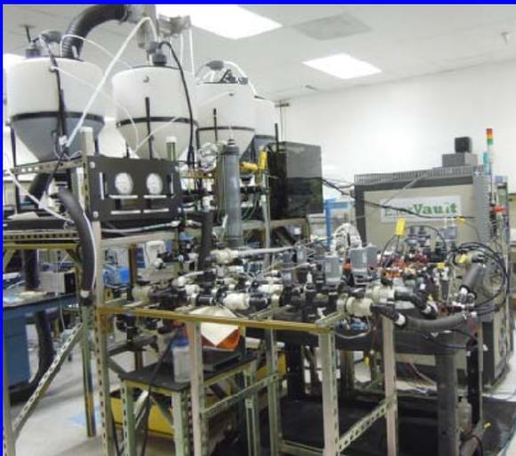
Flow Battery Prototype
