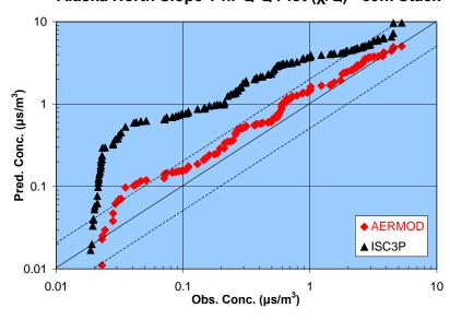
The Q-Q plot for the AGA experiments is shown in Figure 16. This plot shows that the AERMOD predictions parallel the 1:1 line over a larger concentration domain than the ISC-PRIME predictions. For subsets of the modeling cases, AERMOD shows a significant improvement especially for the cases involving stack-to-building height ratios greater than 1.25. Residual plots of prediction concentrations as a function of stability indicate consistently less biased AERMOD results over all stability types.
