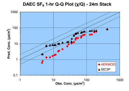
**Figure 14.** Q-Q Plot for DAEC 1-Hour Averages for 46-m Releases (SF<sub>6</sub>)
