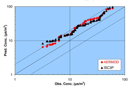
**Figure 11.** Q-Q Plot for Millstone 1-Hour Averages for 46-m Releases (SF<sub>6</sub>)
