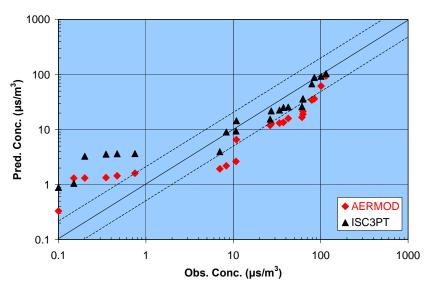
The modeling results for the buoyant releases at the Alaska North Slope experimental site are shown as a Q-Q plot in Figure 15. The AERMOD predictions are nearly unbiased (but slightly conservative), while the ISC-PRIME results are more than a factor of 2 high except for the highest predictions. This result shows some of the biggest performance differences between AERMOD and ISC-PRIME among all seven downwash evaluation databases.
