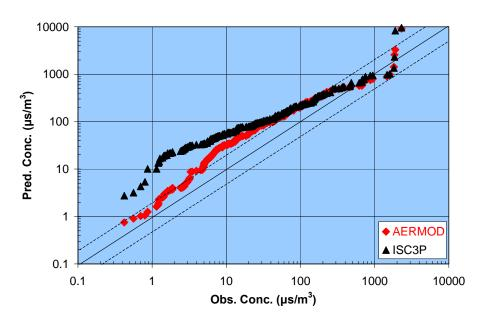
The combined stable and neutral case Q-Q plot for the Lee power plant wind tunnel experiments is shown in Figure 18. This figure shows underpredictions for the peak concentrations, in contrast to the EPRI evaluation results<sup>38</sup> with urban source characterization.
