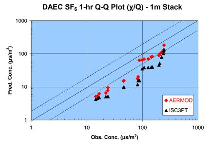
**Figure 13.** Q-Q Plot for DAEC 1-Hour Averages for 24-m Releases (SF<sub>6</sub>)
