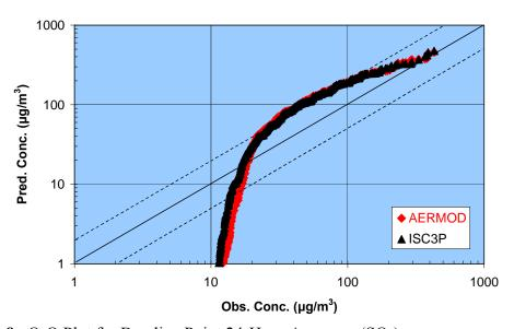
**Figure 9.** Q-Q Plot for Bowline Point 24-Hour Averages (SO<sub>2</sub>)
