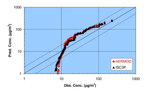
Both models also had a similar evaluation outcome for two non-buoyant release heights (with two different tracer gases) at the Millstone Nuclear Power Plant. Figure 10 shows that both models overpredict by close to a factor of 2 for the 29-m Freon releases, but underpredict by about a factor of 2 for the 46-m SF<sub>6</sub> releases (see Figure 11).
