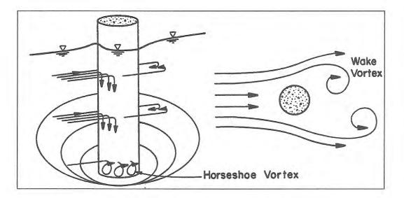
Figure 6. Interference to flow by a pier (After Federal Highway Administration, 2006) The scour hole shaped like an inverted cone changes in size with the flow, it normally
