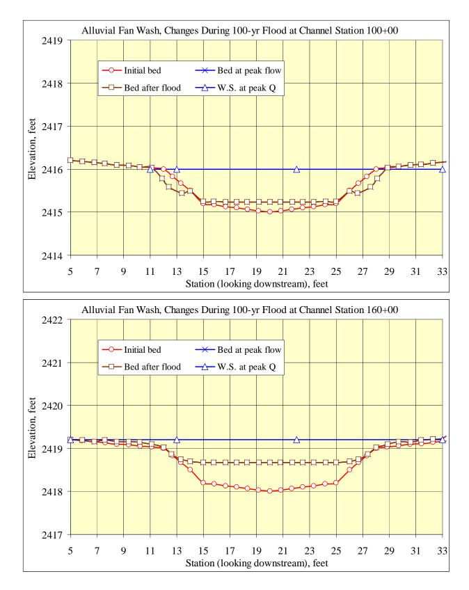
Figure 13. Simulated changes for sample channel cross sections
