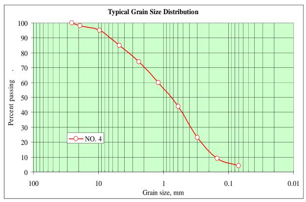
Figure 3. Grain size distribution of sediment sample
