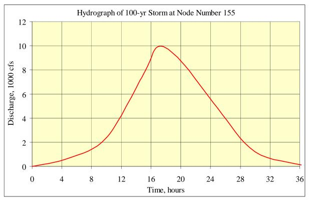
Figure 4. Typical hydrograph of the 100-yr flood at the project site
