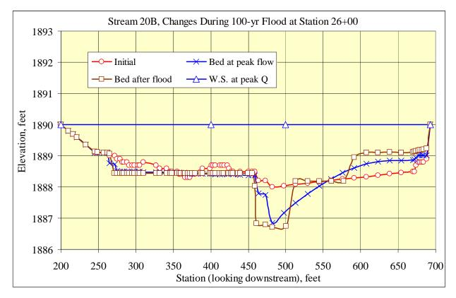
Figure 31. Simulated cross sectional changes at sample cross sections along steam 20B
