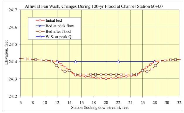
Figure 12. Simulated changes for a sample channel cross section
