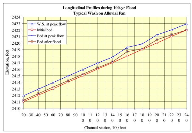
Figure 11. Water-surface and channel bed profile changes during 100-yr flood for sample wash
