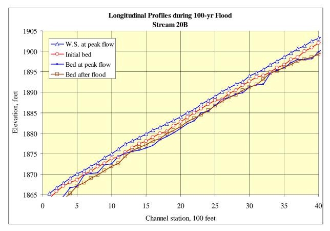
Figure 30. Water-surface and channel bed profile changes during 100-yr flood for stream 20B
