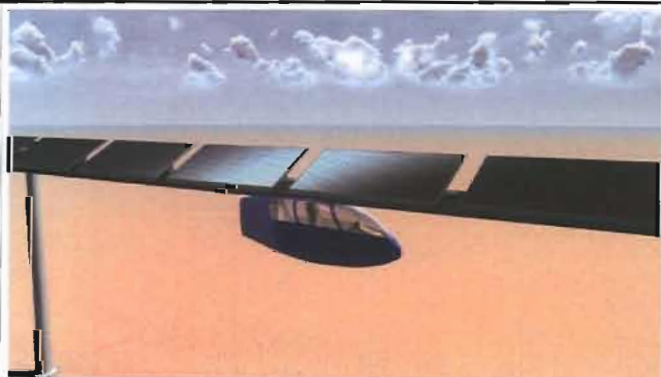
A contiguous 24-inch wide solar panel on a SkyTran guideway can supply all the power necessary to move 3,600 vehicles per hour at 35 mph (above). SkyTran portals use an electric lift to provide ADA access for disabled passengers (right).
