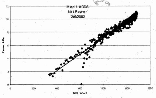
Fig. 16 Mod 1 ADD system net power output versus direct normal insolation
