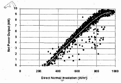
Fig. 9 SBP system net power output versus direct normal insolation
