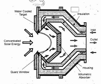
Fig. 18 DLR pressurized volumetric air receiver
