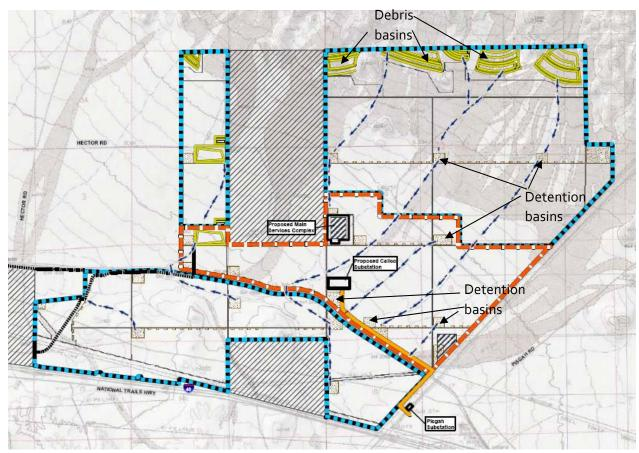
Figure 23. Detail from applicant's proposed drainage plan showing the debris basins (green blocks) and detention basins (brown blocks). Source: URS, 2010.
