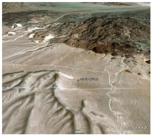
Figure 27. Oblique aerial photo of Off-Site Area 2. Source of sediment is not as clear as for Area 1, but appears to be the local washes rather than the project site (located almost 4 miles to the west).
