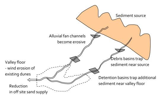
Figure 24. Conceptual response of geomorphic system to the proposed drainage plan
