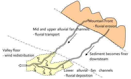
Figure 4. Conceptual model of sediment transport processes supporting dunes
