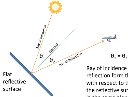
Ray of incidence and ray of reflection form the same angle with respect to the normal of the reflective surface and are in the same plane
