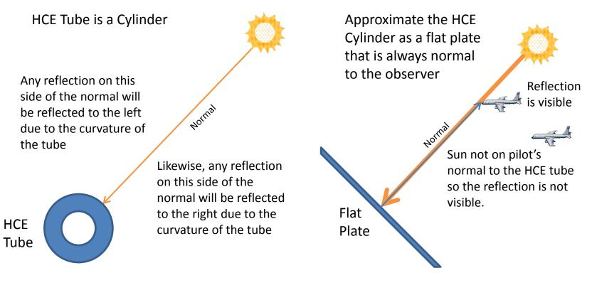
The strongest reflection that an observer can see is from the point normal to the cylinder with respect to the observer The pilot will experience the strongest reflection only when the HCE tube, the pilot, and the sun are all in a direct line.
