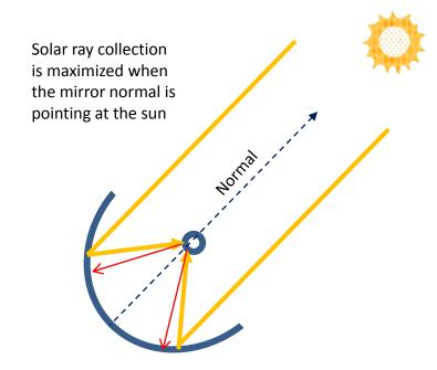
Maximum outgoing intensity is along the line of the normal to the HCE tube/mirror.
