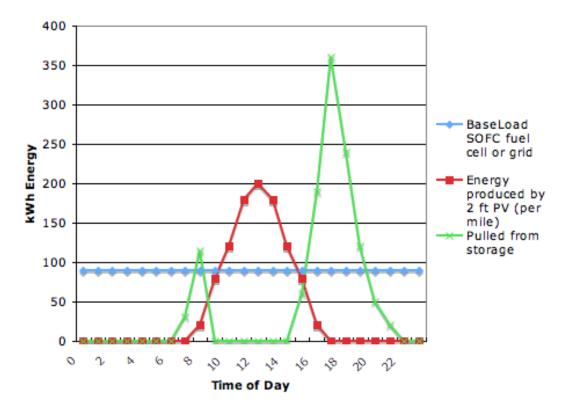
FIGURE 2 Example MPRT system with 30,000 daily ridership requiring 3,156 kWh energy per day, combined with 1,000 kWh of PV and 2,156 from a SOFC fuel cell and 1,156 kWh storage system.
