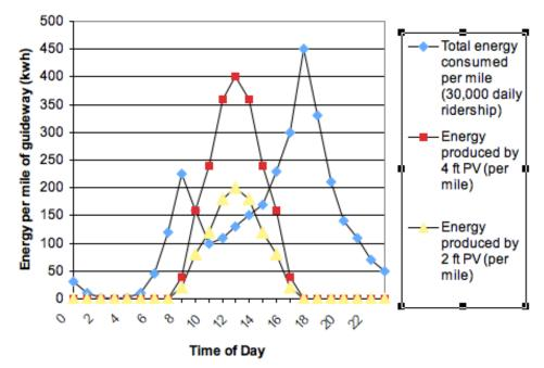
**FIGURE 1** Production and consumption of energy in a solar-powered MPRT system.
